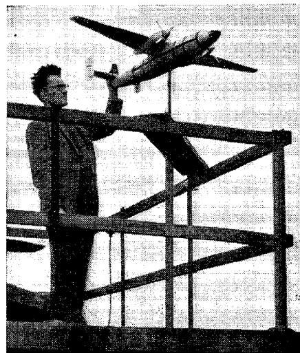
Fig. 5. Scale model aircraft used for polar diagram measurements.
